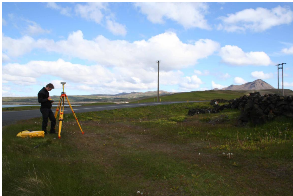
Fig.2 Setting up DGPS base-station at Hlidarétt near Reykjahlid
