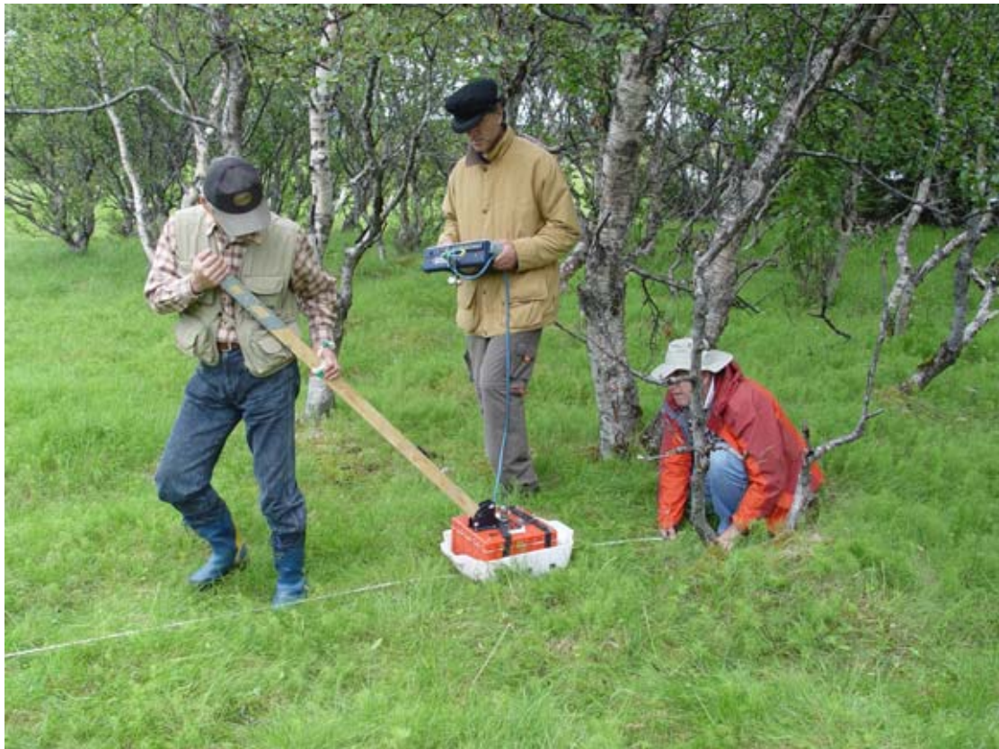
Fig. 1. GPR surveying with 400 MHz antenna. Dean Goodman on console, Yasushi Nishimura towing antenna and Antonio Gilman with measuring tape.
