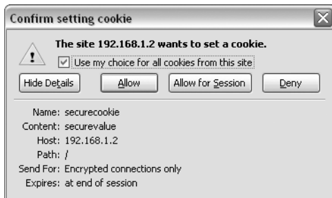
Figure 11-16. A dialog box indicating that a cookie with the secure flag was sent
